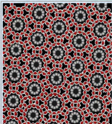
Fig. 1. 0.4nm SWNTs array in the channels of zeolite AFI single crystal, viewed along (001) direction.
